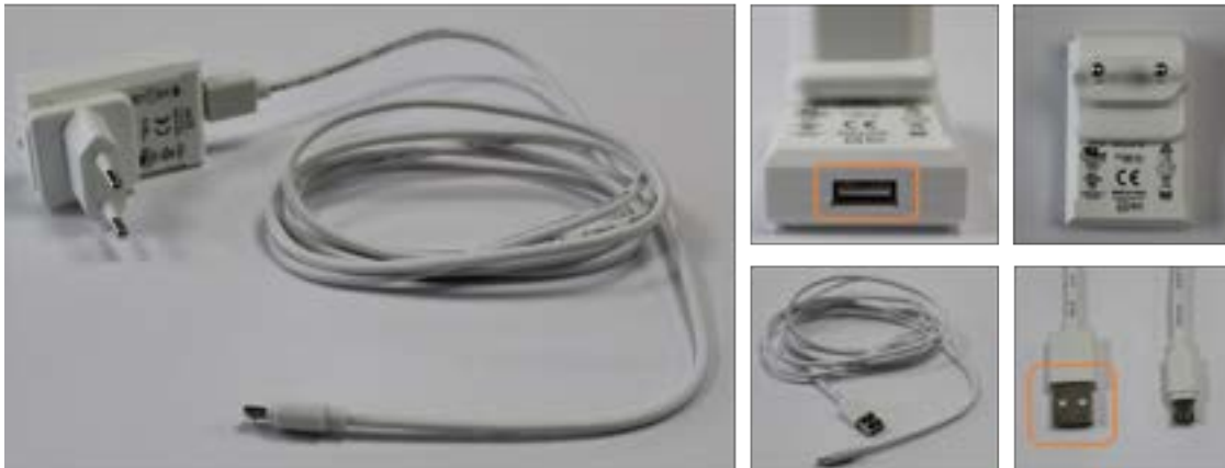
Figure 3-3: PainSensor power supply
